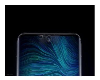
It integrates a small rectangular area into the phone's display which uses a "special low-reflective glass with high transmittance." The front-facing **camera** sits **underneath**. It allows the **screen** to display imagery unhindered, but at the same time doesn't block light reaching the **camera** when in use.
